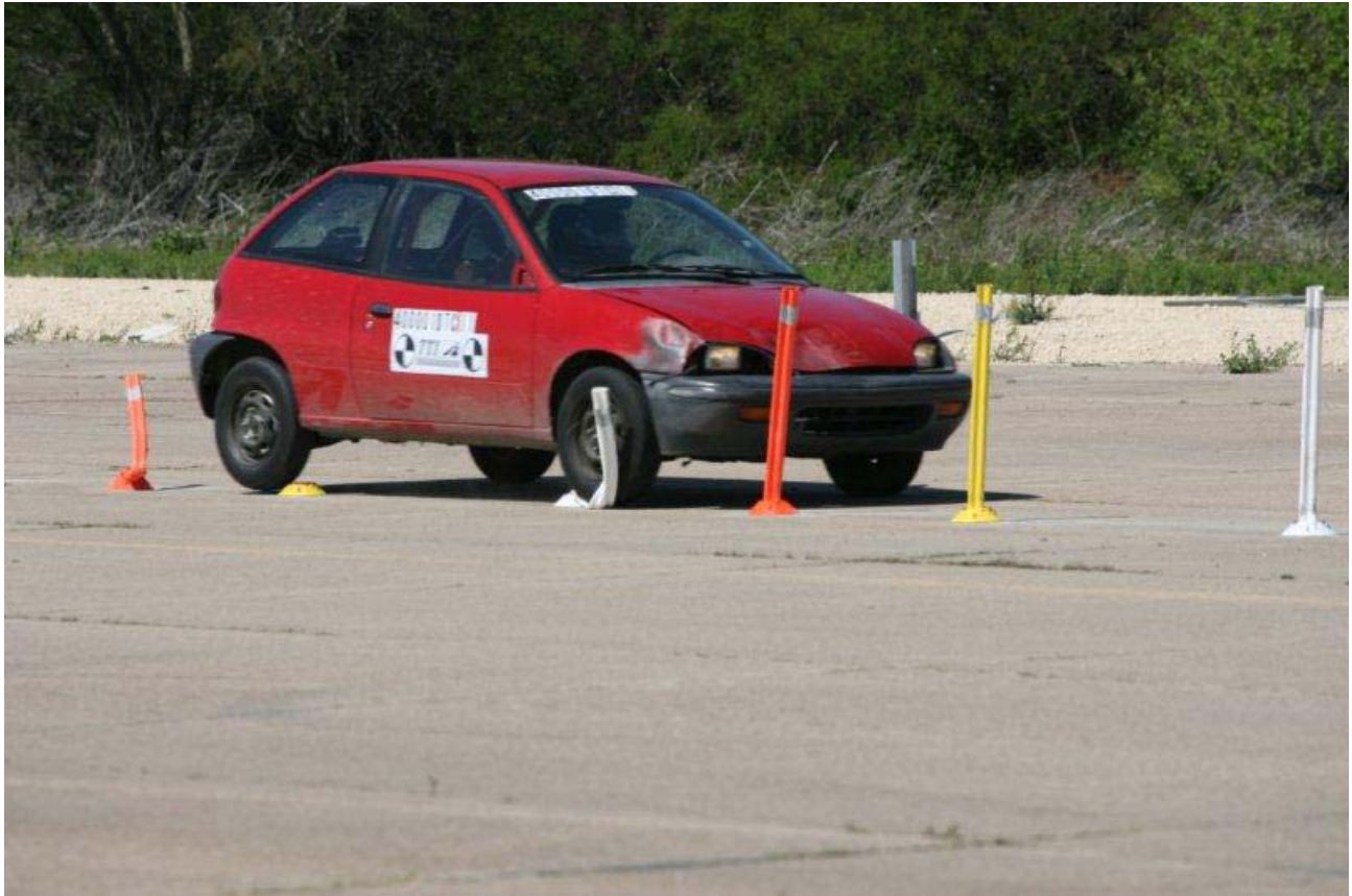
Davidson FG 300 Model UR Posts Survived 50 High Speed Impacts at 60 MPH
