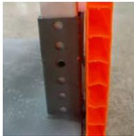
B) The bottom panel of the TPAR barricade requires only one bolt, nut and nylon spacer inserted into the top hole. This allows for the assembly to slip easily into the foot and be under maximum ADA height.
