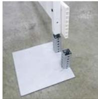
C) For a continuous run, position the steel foot with the base plate pointing away from the pedestrian walkway. Then simply slide the bottom of the X-tube post into the steel foot and repeat on the other side.
