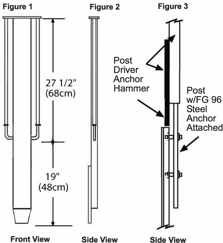
1. Place the delineator post with steel anchor attached into the FG 103 Driver. See Figure 3 to the left.
