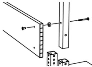
b) Apply the washer to bolt threads as shown
