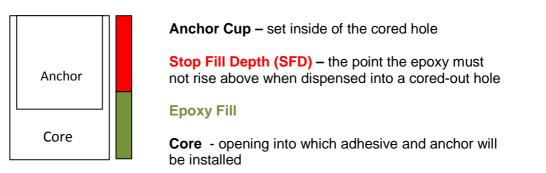
**For example:** using a 2.25" core the adhesive can reach a maximum fill that leaves 1.61" of air space. The air space will be displaced by the anchor cup when inserted.
