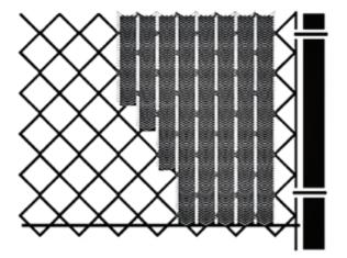
These Insert HedgeLink Slats vertically top to bottom, keeping the green needles facing up, while revolving the slat clockwise with your fingers for easier installation.
