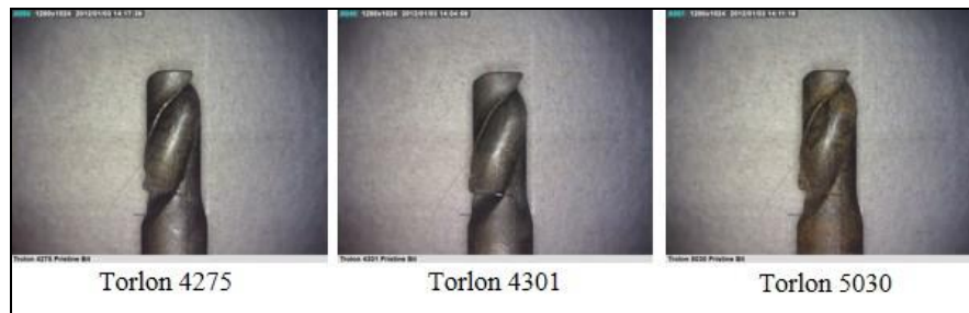
Figure 22. Pristine Torlon GRF-Bits
