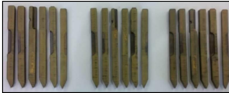
Figure 44. Sectioned Injection Molded TSBs
