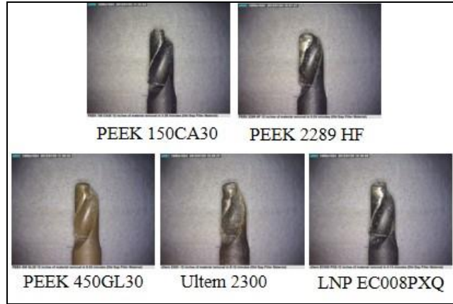
Figure 20. GFR-Bits after Removing Old Gap Filler
