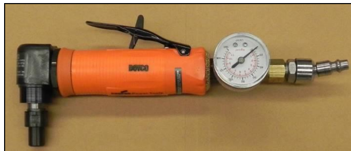
Figure 13. Dotco (20,000 rpm) 90-degree Grinder with Regulator
