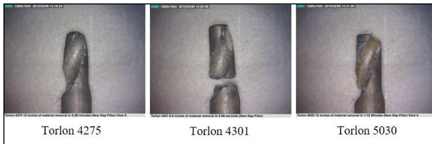
Figure 24. Torlon GFR-Bits after Removing New Gap Filler
