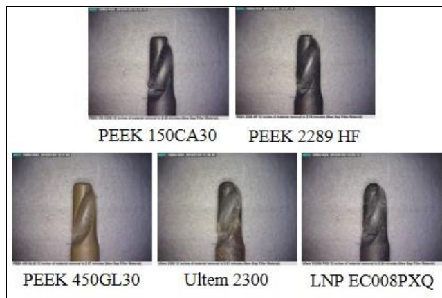
Figure 21. GFR-Bits after Removing New Gap Filler
