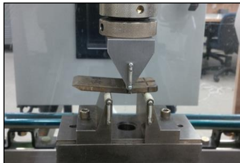
Figure 45. TSB Three-Point Bend Test Setup
