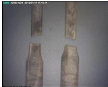
Figure 15. Typical Failure of Straight Single and Double Flute GFR-Bits
