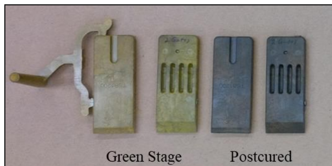
Figure 43. Injection Molded TSBs (TSB-1200)
