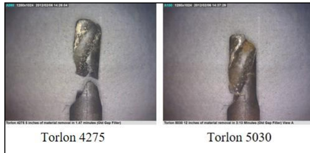
Figure 23. Torlon GFR-Bits after Removing Old Gap Filler
