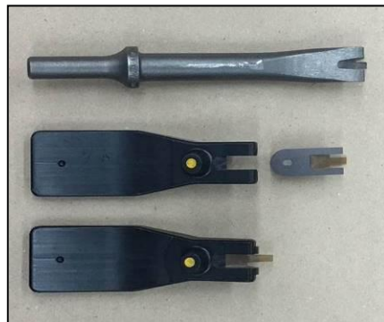
Figure 65. Sheet Metal Ripper with Prototype TGBs and Adapters
