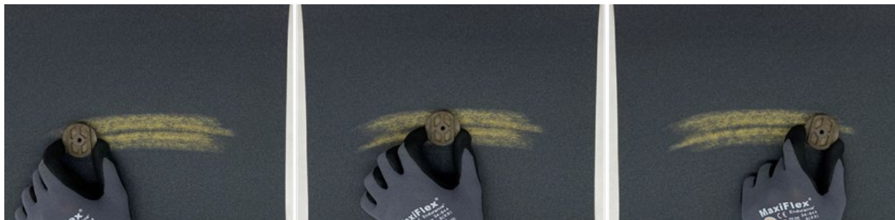
Figure 15. Restoration of the Cutting Surface of the Torlon Adhesive Cutter
