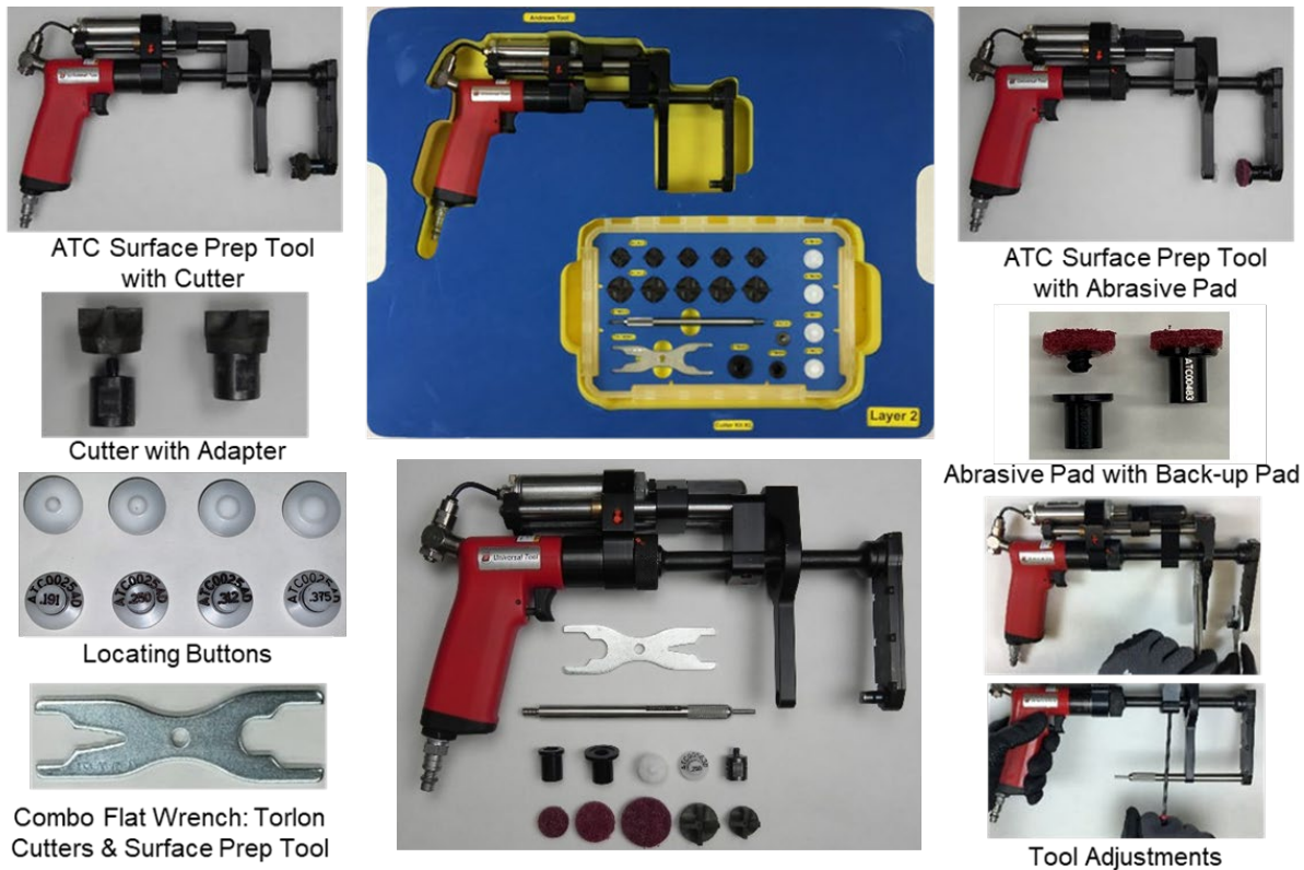
Figure 9. Surface Preparation Kit – Layer 2: ATC Surface Preparation Tool and Associated Tools in Various Configurations
