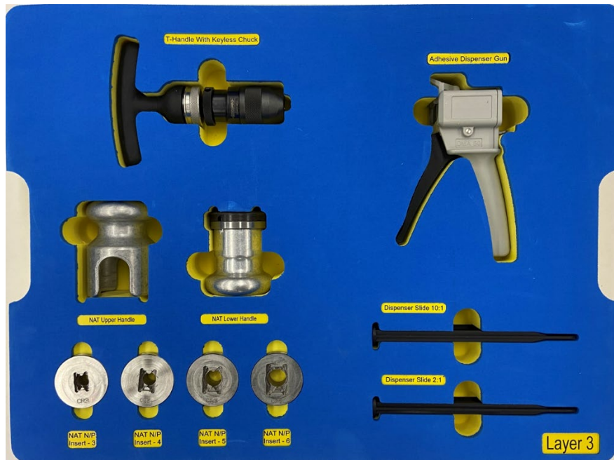
Figure 4b. Surface Preparation Kit – Layer 3: T-handle, Nutplate Abrasion Tool (NAT) with Inserts and Adhesive Dispensing Gun with Slides
