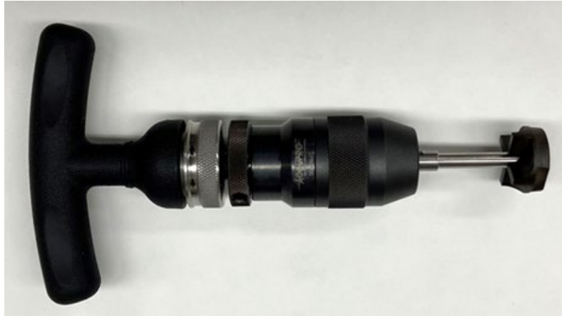
Figure 18. T-Handle with Torlon Adhesive Cutter for Removal of Bulk Adhesive/Sealant
