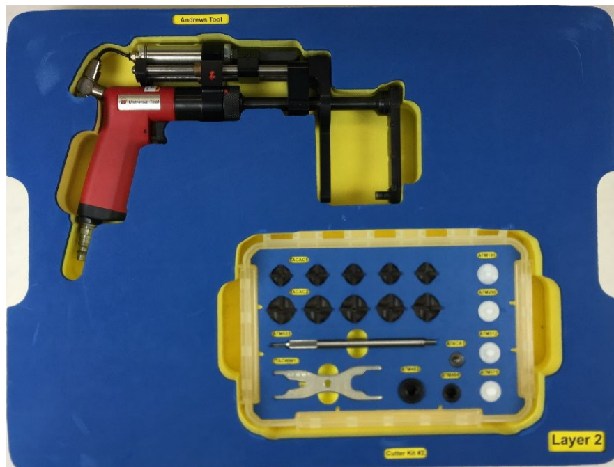
Figure 3. Surface Preparation Kit – Layer 2: ATC Surface Preparation Tool & Associated Torlon Adhesive Cutter Kit
