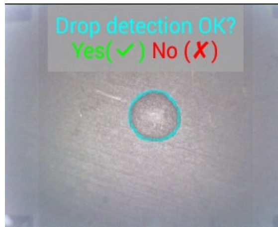
Figure B-7. Example of Acceptable Drop Detection
