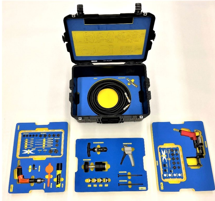
Figure 1a. Surface Preparation Kit – Tools for Bulk Adhesive/Sealant Removal and Final Structure/Nutplate Surface Preparation – with Rotary Abrasion Tool (RAT)
