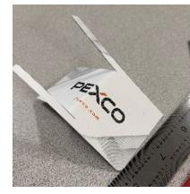
The flap of the card should match the stop fill depth required. When filling the core hole with epoxy, stop as soon as contact is made with the edge of the flap that is inserted into the hole.
